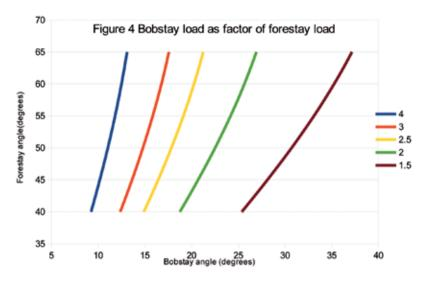
That gives us just over 13 tonnes compression in the bowsprit. Note that even on an 8 tonne boat with a moderate bowsprit, we have bowsprit and bobstay loads a good deal greater than the displacement of the boat.
